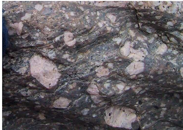
Figure 3. Porphyritic texture, in which euhedral feldspar phenocrysts are surrounded by finer-grained material.
